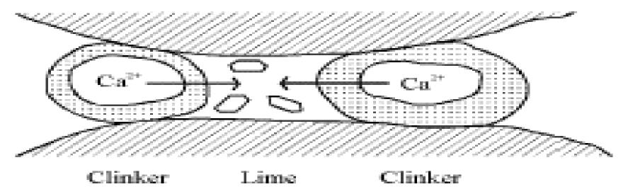
• 7: The pore filling of Portland cement concrete
