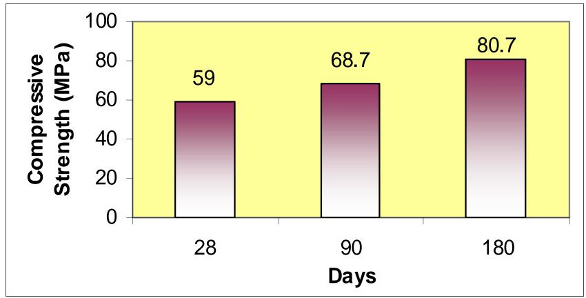
Increase in strength at 180 days is 36% higher than at 28 days
