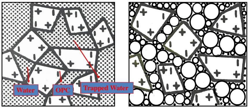
Presence of electronic charges, on Portland cement particle surface, tend to form flocks that trap large volumes of water "Dispersion of Cement Particles" - Fine HRS particles get adsorbed on the oppositely charged surface of the cement particles and prevent them from flocculation
