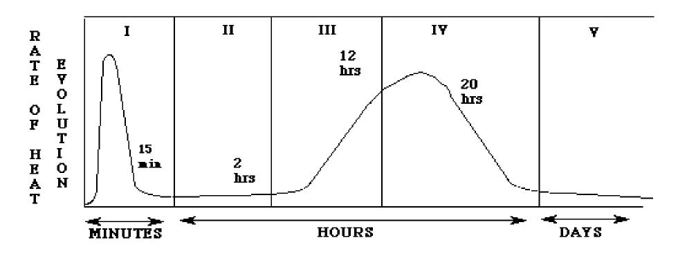
Liberation of Heat is linked to chemical activity, this further affects hardening process. Please note the high exothermic activity at start, gypsum cooling and exothermic activity close to final setting.
