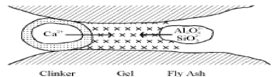
9: The pore filling of fly ash cement concrete
